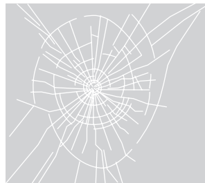
< Broken Laminated Glass >
